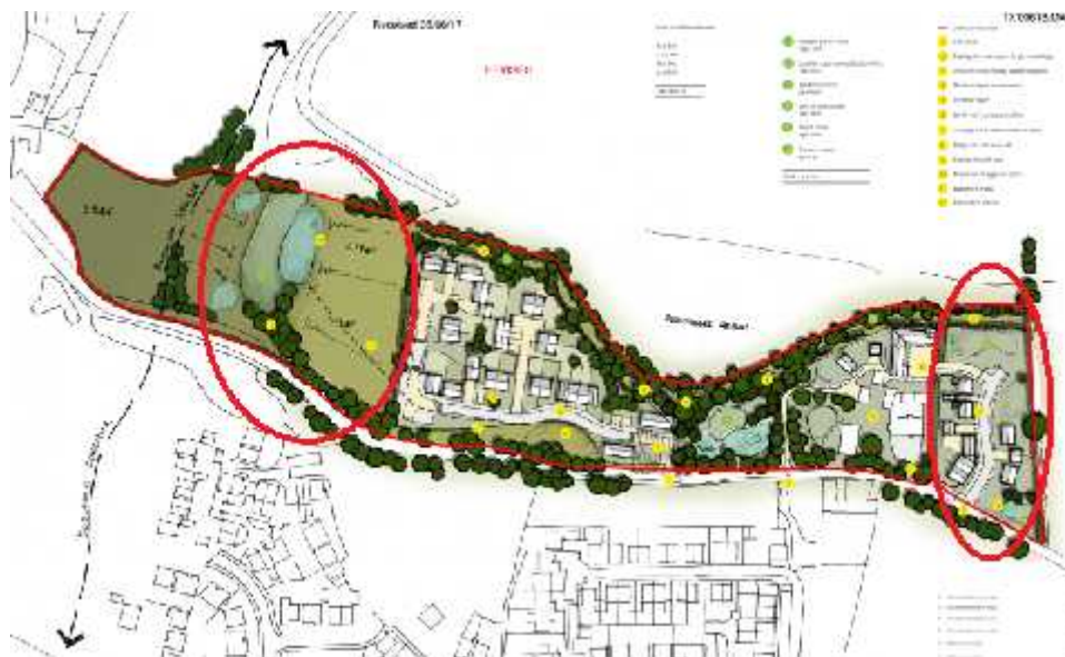
Figure 2: Illustrative Site Layout as submitted by the applicant illustrating how the development areas have swapped due to the topography of the land.
